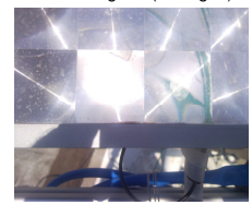
Figure 8 Soiling effect on the lenses (I-V), (P-V) curves of the Solartec module, which introduced a Mr(1) value of 15%.
