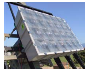
16.4% eff DNI Power 840 W, Tcell= 40°C (eff 17.8 % lens parquet apertura area)
